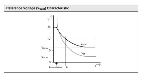
After  $t_{bl}$  has passed, the V<sub>CE</sub> monitoring will be triggered as soon as V<sub>CE</sub> > V<sub>CEref</sub> and will turn off the IGBT. The error memory will be set, and the output PRIM\_nERROR\_OUT changes to the HIGH state. Possible failure modes are shows in the following pictures.
